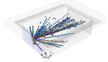
The figure shows the ionization in the TPC for event. The beam initially travels in the Z direction and strikes a target located approximately 1 cm upstream of the TPC.
